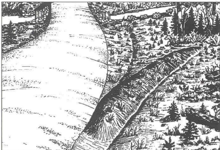
A diversion ditch into a filter area is a good alternative to a water bar or cross drainage culvert where slope allows.
